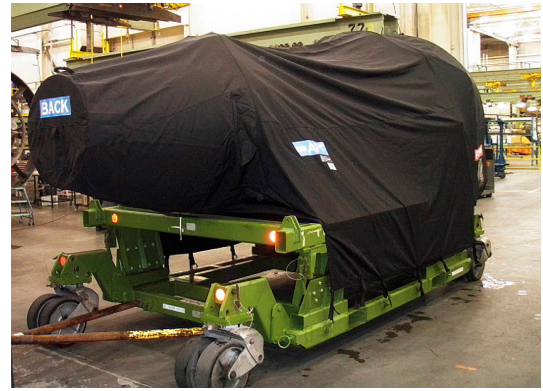
PW 2000 Series OFF-LINK ENGINE STORAGE COVER, Rain Cap
