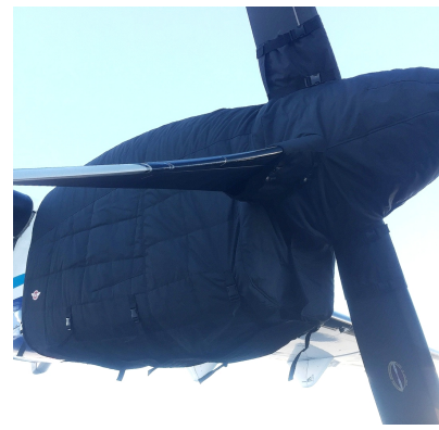
ATR-72-202 Insulated Engine & Prop Hub Covers
