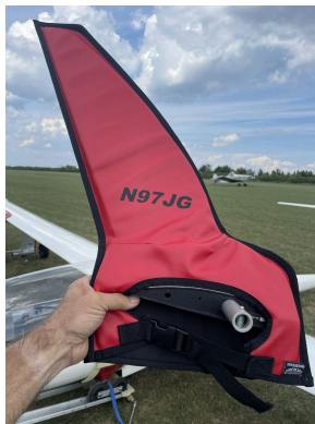
Schempp-Hirth Ventus-2B winglet/wingtip pads
