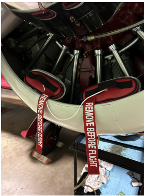
Beech Staggerwing Carb Inlet Plugs, Located Inside Engine
