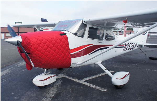
Cessna 172 Insulated Engine Cover, fully enclosed
