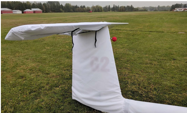
SZD Jantar Empennage Cover Set, test fit covers
