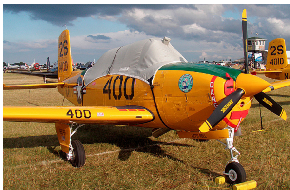
T34 Canopy Cover & Engine Inlet Plugs
