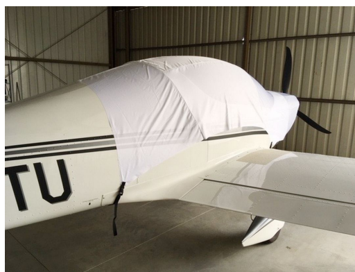
Tecnam Astore Canopy/Engine Cover, test fit cover
