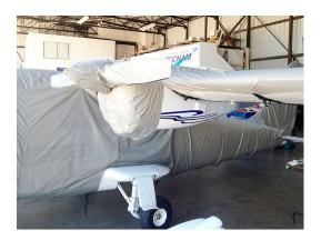
Tecnam Twin Canopy/Nose, Empennage, Wing/Engine, & Propellor/Spinner Covers
