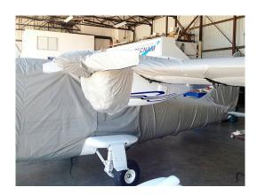
Tecnam Twin Canopy/Nose, Empennage, Wing/Engine, & Propellor/Spinner Covers
