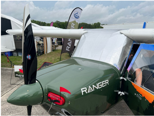
Vashon Ranger VR-7 Engine Plugs, Windshield HeatShield
